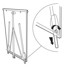
Rotate the back leg until the triangular brace reaches the locking mechanism, then release the bottom section of the back leg, angle the easel to its desired position and retighten.
