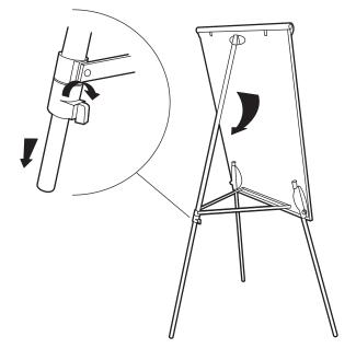
To load the flipchart pad, simply lift the top clamp, slide the hooks into the correct position for your pad, hang the pad and close the clamp.
